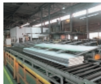
A production line for rigid polyurethane thermal insulation panels
