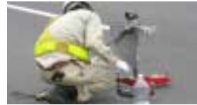
Slippage resistance measurement
