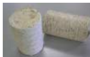
Rigid polyurethane board material remnants after being compressed to reduce volume
