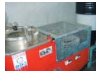
Waste Solvent Collecting Machine Collected solvents are reused for cleansing painting hangers.
