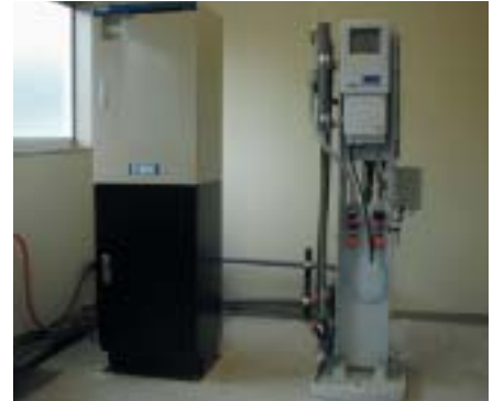
Left: Automatic nitrogen and phosphorus measuring system Right: Automatic COD measuring system
