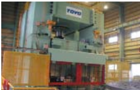
Large-scale horizontal rigidity testing system
