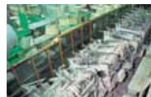
Automotive polyurethane seat cushion manufacturing line using improved heat-retaining molding
