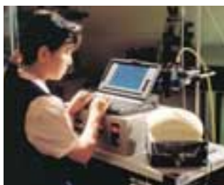
Measurement of polyurethane foam hardness
